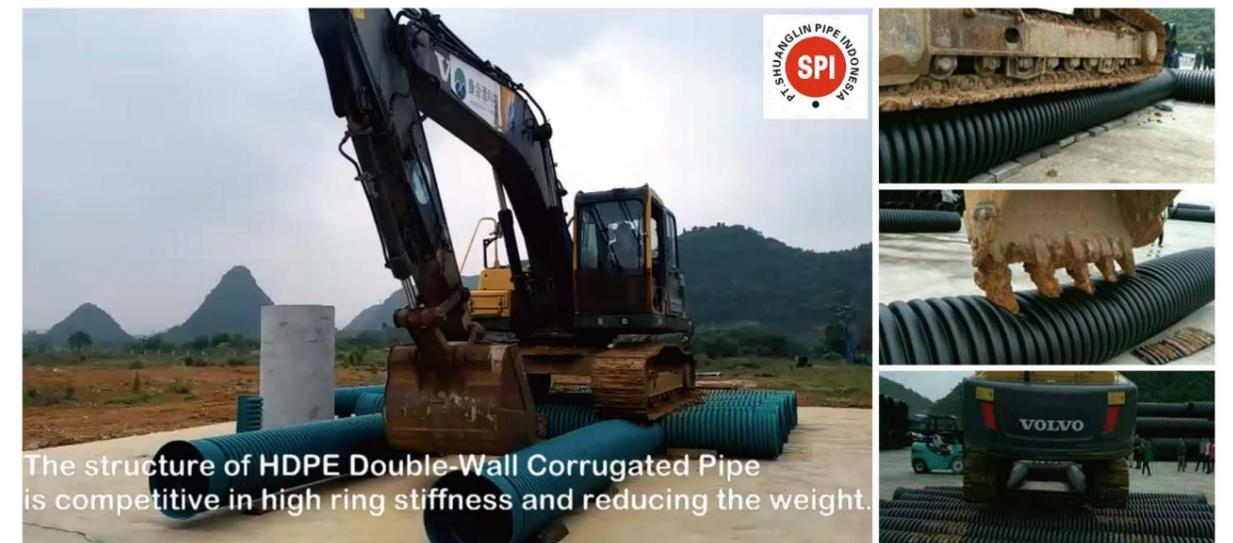
The structure of HDPE Double Wall Corrugated Pipe is competitive in high ring stiffness and reducing the weight.
